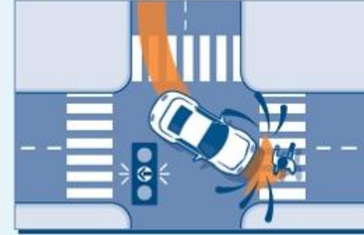
Left Turn Crash at Signalized Intersections
